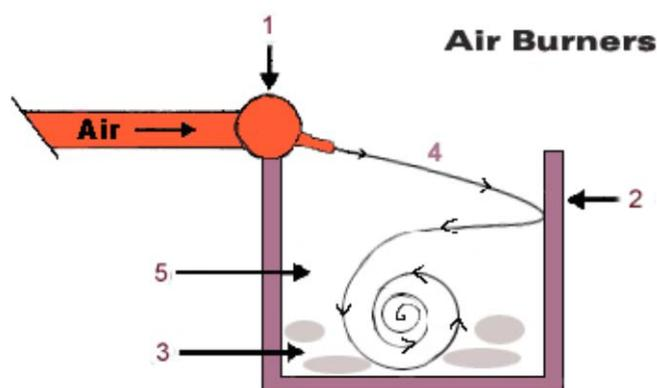
1. Air curtain machine manifold and nozzles direct high-velocity airflow into refractory lined firebox or earthen pit.
