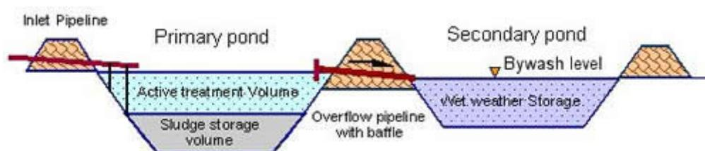
**Figure A9.2** Cross-section of double effluent pond, showing location of storage volumes in each pond
