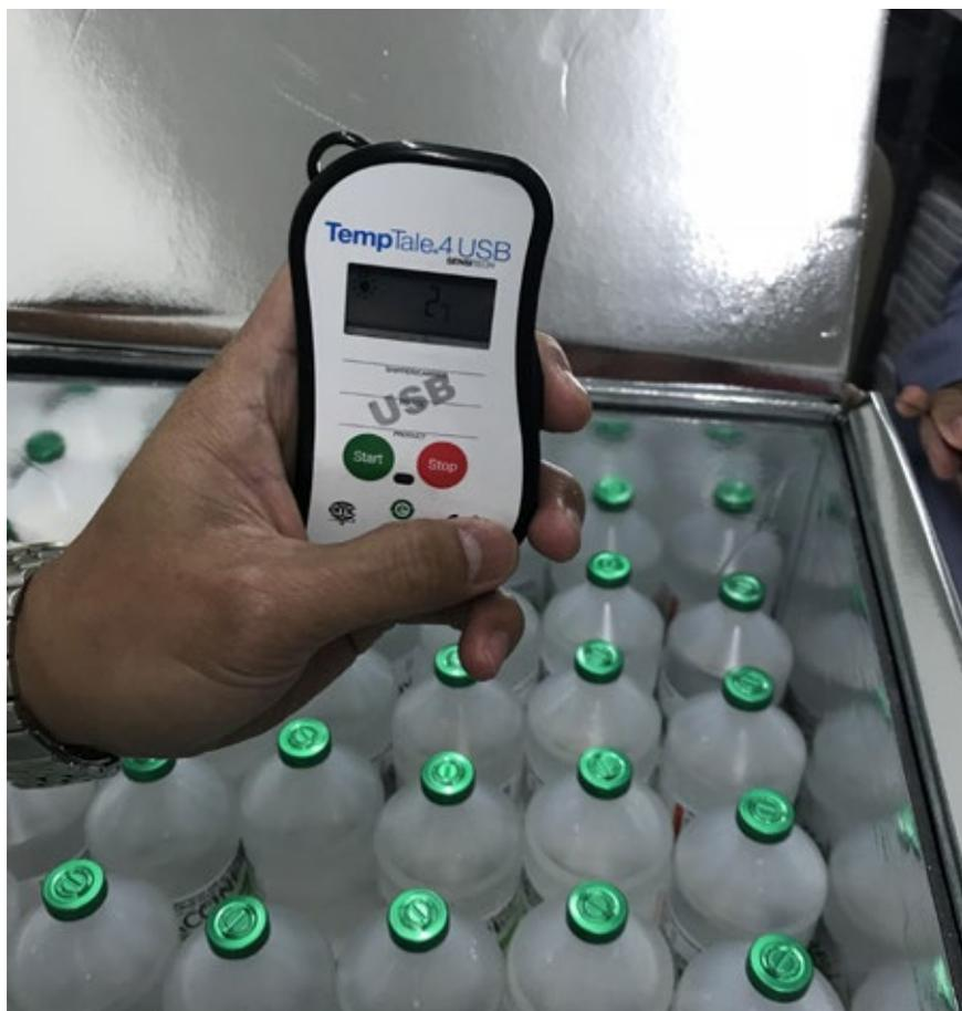
Checking the temperature of the test consignment of simulated FMD vaccine on the internal USB data logger.
